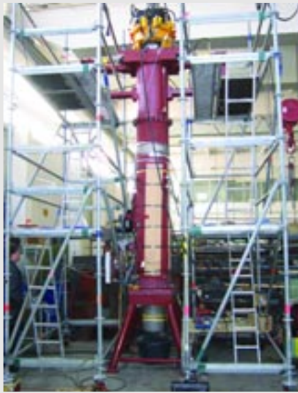
Leak Tightness Test at DSI Laboratory
