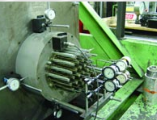
Anchorage of a Fatigue Test
