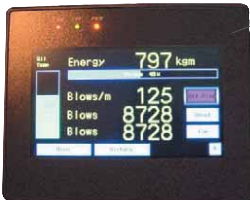
INTERFACE SCREEN MOUNTED ON POWER PACK
