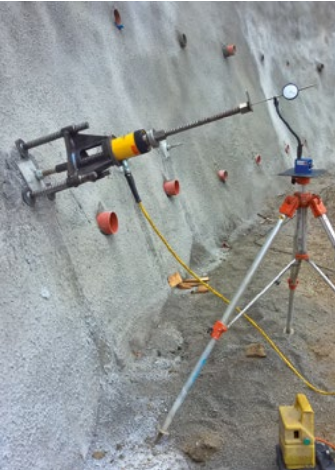
In-Situ Pull Testing (DIN 21521-2): Load-Displacement Diagram R32-360 with DYWI® Inject SILO 8044-M
